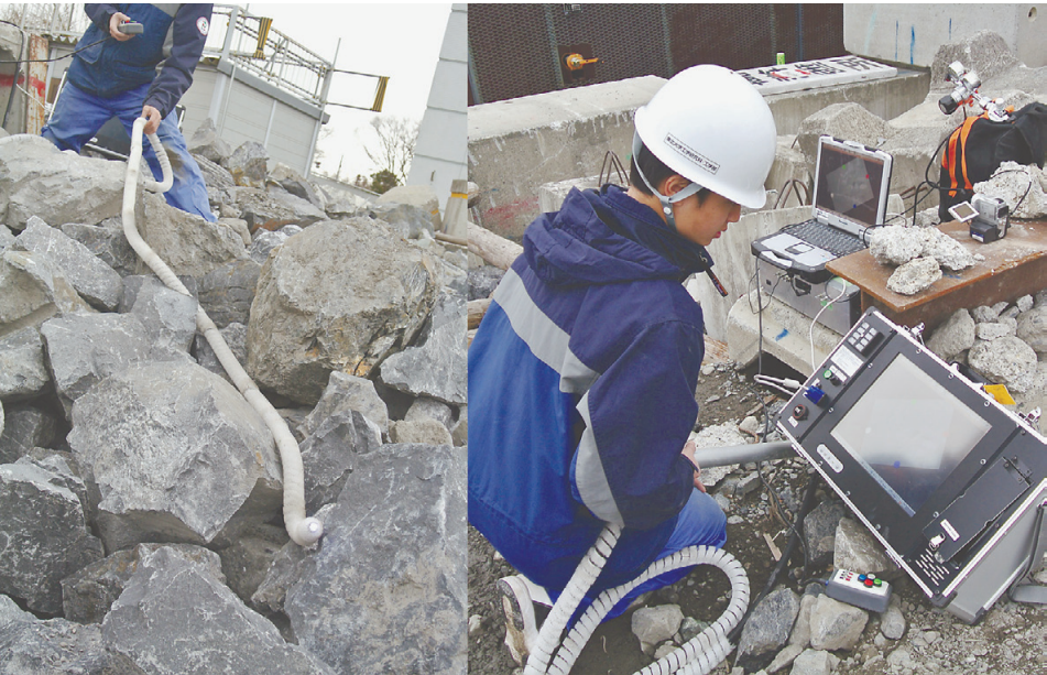
The Active Scope Camera is a fiber-optic scope that seeks out tiny cracks rescuers would be unable to explore. HUMAN-ROBOT INFORMATICS LABORATORY
