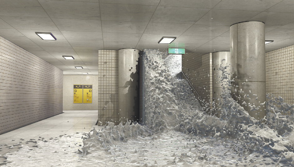
An image created by “Particleworks” software shows a prediction of how flood waters will move. PROMETECH SOFTWARE INC./KOZO KEIKAKU ENGINEERING INC.
