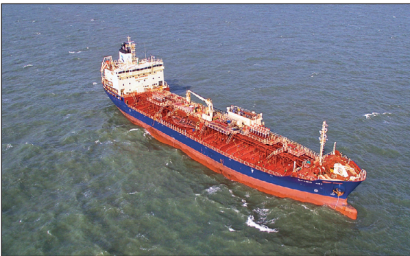
Nordic Tankers pursues highly specialized, quality ships built in Japan. One of the company's chemical tankers, the Nordic Aki is 14,701 DWT with 28 segregations, and was built by the Fukuoka Shipbuilding Company.
