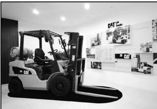
The Cat Lift Trucks model GP25T has a lifting capacity of 2,500 kg and is equipped with an LPG system.
