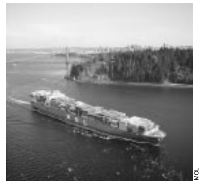
Hirokazu Hatta, managing director of Mitsui O.S.K. Lines Australia (above left). Completed in 2003 by Mitsubishi Heavy Industries in Japan, the Efficiency (above) has a capacity of approximately 4,600 TEU (Twenty-foot equivalent) with a gross tonnage of approximately 53,000. It is 294 meters long and 32 meters wide.
