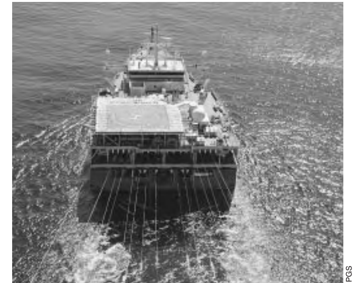
The purpose-built Ramform vessels of PGS can tow up to 20 streamer lines, allowing a more extensive and accurate survey of the ocean floor.
