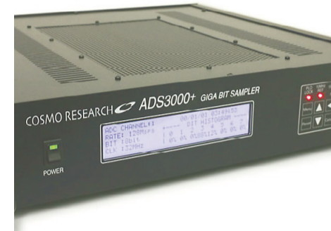
Clockwise from top left: A satellite command antenna made by Antenna Giken; Components used in medical endoscopes, machined by Kaneko Manufacturing Co.; A steel plate, used in LCD-making equipment, being dried at Nishina Industrial Co.; An ADS3000, equipment sampling electric wave from stars, made by Cosmo Research Corp. SAITAMA CITY
